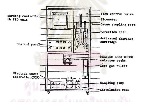
Figure A-1 Ozone automatic control recorder
