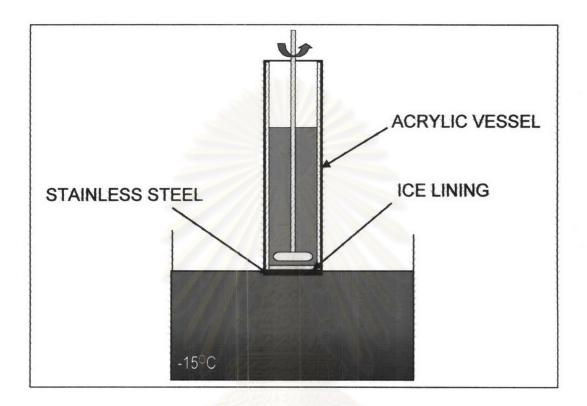
Fig.3.6 The beginning of progressive freeze-concentration experiment
