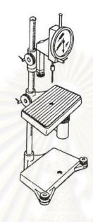
Figure 3.1 Penetrometer
