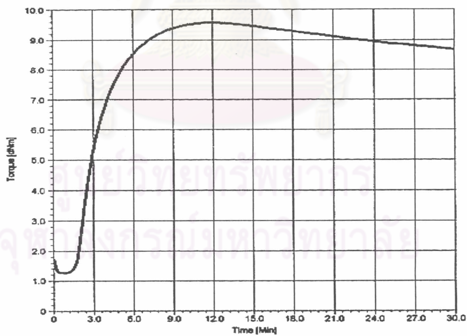
Figure C.4 A vulcanization curve of compound B2.
