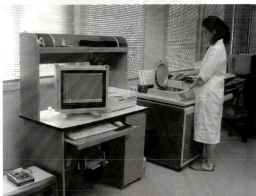
Figure 5.1 Energy Dispersive X-Ray Fluorescence Spectrometer (EDXRF) at GIT was used to analyze trace composition in Songea corundums.
