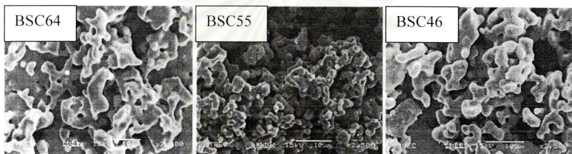
Figure 4.23 SEM pictures of top view of BSCF 5582 membrane coated by BSC 64, BSC 55, and BSC 46 sintered at 1,000 °C, 5h.
