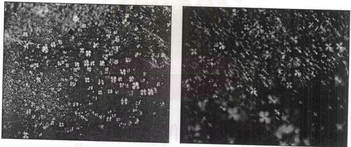
Figure 40 The microscopic pattern under cross-polarized light microscope showing the birefringent property of system (6/4) IPM:T 80 :C EL :W (20%), (IPM:T 80 :C EL =1: 4.5: 4.5) exhibited lamellar phase structure (left: 40X and right: 100X crossed polars).
