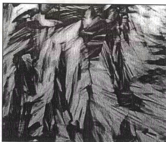
Figure 42 Typical hexagonal liquid-crystalline texture formed by heptane: non-ionic surfactant and water system (from Cordobes et al, 1997).
