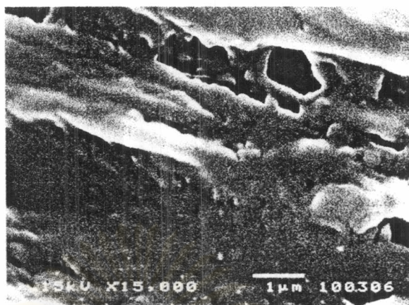
Figure 28: Scanning electron photomicrograph of the cross section of cellulose acetate film plasticized with 23.08 %w/w of PEG 400 in polymer after dissolution test for 12 hours (X15,000).
