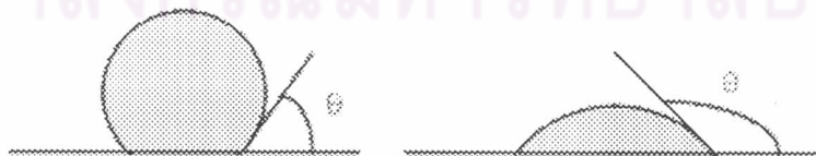
Figure 2.1 A liquid droplet in equilibrium with a horizontal surface surrounded by a gas.
