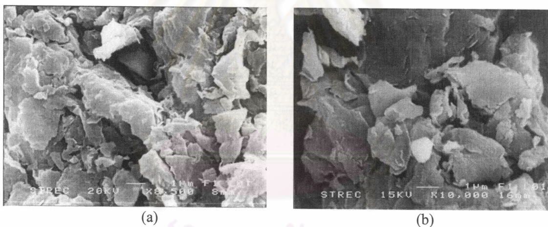
Figure 4.10 SEM images of hectorite (a) and HFe_{10} (b).
