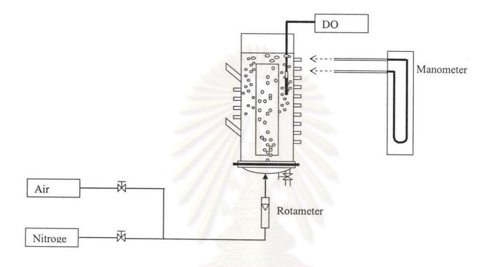
Figure 3.1 Experimental setup of the internal loop airlift contactor
