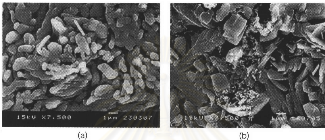
Figure 4.34 SEM micrographs of the film microstructures gained from DCPD electrolyte based 1 M- \text{H}_3\text{PO}_4 solution at -300 \text{ mA/cm}^2 for deposition time of (a) 7mins and (b) 10 mins.
