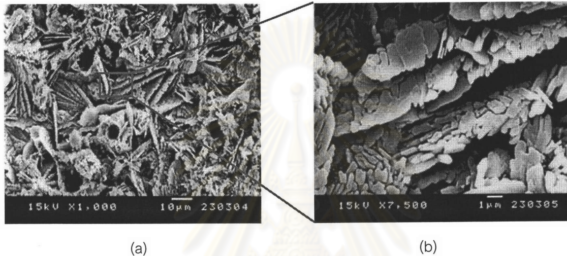
Figure 4.4 SEM micrographs calcium phosphates film gained from MCPM based aqueous electrolyte at -10 \text{ mA/cm}^2 for 3 minutes at (a) 1,000x and (b) 7,500x respectively.
