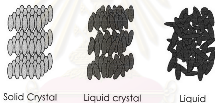
Figure 12 Arrangement of molecules in solid crystal, liquid crystal and liquid
