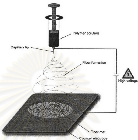
Figure 1 Schematic drawing of an electrospinning set-up
