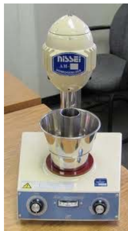
Figure 3.2 Homogenizer for coal-water slurry preparation.
