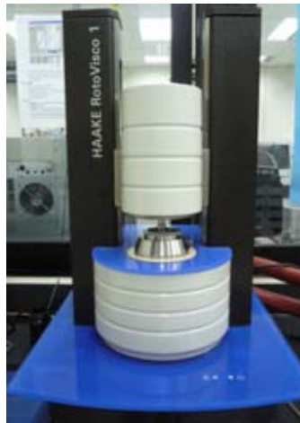
Figure 3.3 HAAKE rotational viscometer (HaakeRotoVisco 1).
