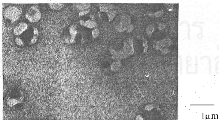
Figure 4.13 TEM photograph of P(DMAEMA- co -ST)/PMMA composite particles (Run 202) prepared by swelling method. [P(DMAEMA- co -ST) domain was stained with RuO 4 ].
