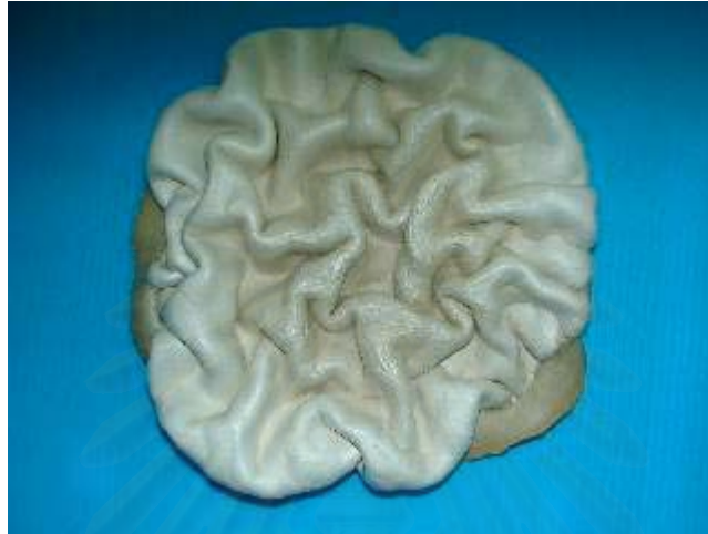
Figure B1 Composite material from natural rubber and 60% sticky rice flour heated by compression molding at 180^{\circ}\text{C} / 15 min.
