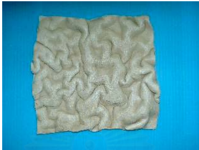
Figure B3 Composite material pressed by compression molding at ambient temperature
