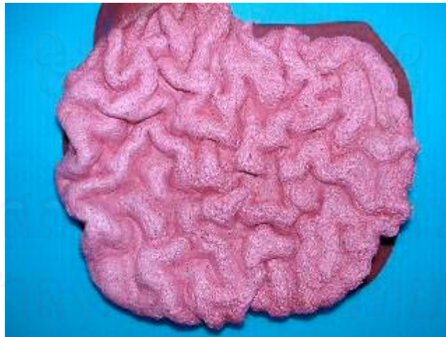
Figure B2 Composite material from natural rubber and 60% sticky rice flour mixed with dye (to test colouring) and then heated by compression molding at 180^{\circ}\text{C} / 15 min.
