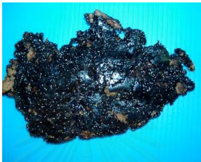
Figure B7 Composite material from natural rubber and 60% sticky rice flour composed of maleic anhydride 10% of flour and benzoyl peroxide 2.5 phr content heated at 180°C/ 15 min.
