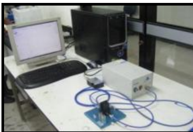
Figure 3.3 The Ocean optics Portable UV-visible spectrometer setup
