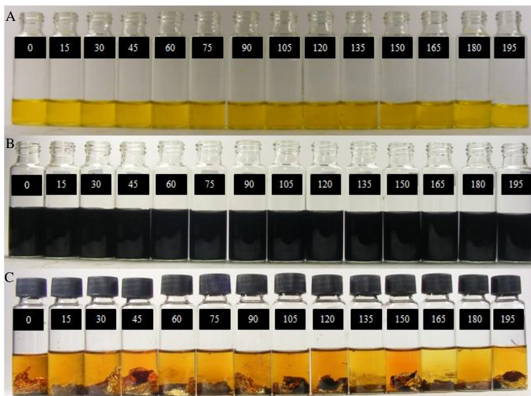
Figure 4.18 Synthesized gold nanopowders reduced by various incubation times between gold ions and soluble starch before the reduction reaction. A: gold ions in soluble starch (part I), B: after part I was mixed with part II immediately, C: after part I was mixed with part II for 3 hours.
