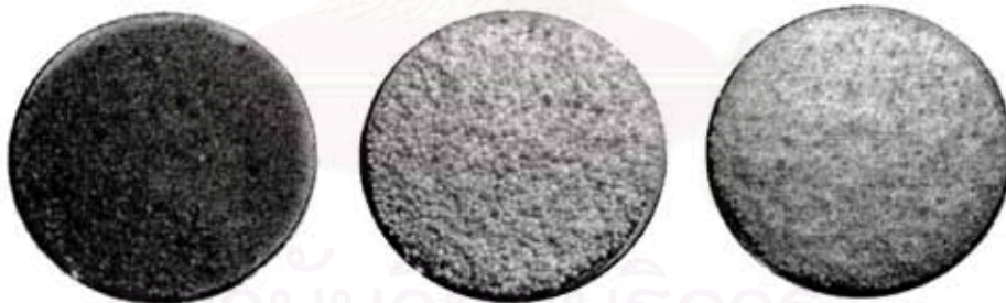
Figure 2.1 Three types of nitrogen source; (a) ammonium sulfate, (b) ammonium nitrate, (c) urea.
