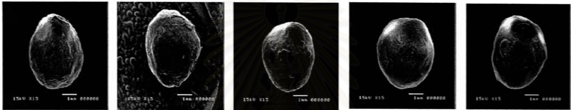
(a) 1 layer coated fertilizer (b) 2 layers coated fertilizer (c) 3 layers coated fertilizer (d) 4 layers coated fertilizer (e) 5 layers coated fertilizer
