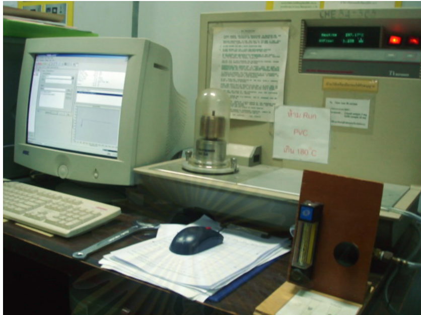
Figure 4.3 Differential Scanning Calorimeter (DSC)
