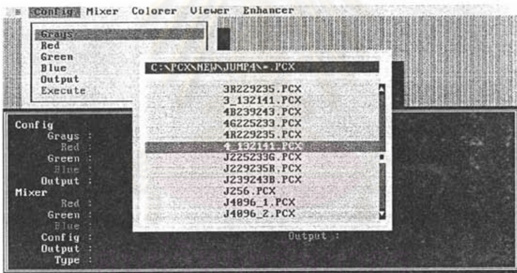
Fig. 4.2 File selection via file list when the file specification contains wildcard character(s)
