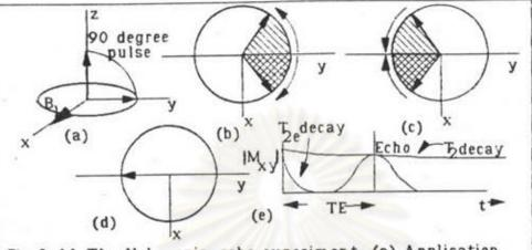
Fig.2-11 The Hahn spin-echo experiment. (a) Application of 90 degree pulse. (b) Dephasing of spins during period TE/2. (c) Position of spin isochromats following 180 degree pulse. (d) Negatively-refocused magnetization after further period TE/2. (e) Evolution of magnetization in xy-plane of rotating frame. Note the sign reversal following the 180 degree pulse has been removed for clarity. (Morris 1986: 49)
