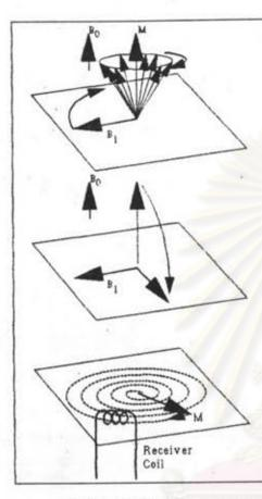
Fig.2-7 Transverse magnetization is produced by a radio frequency field B, rotating synchronously with the precessing spins. (GE: 8)
