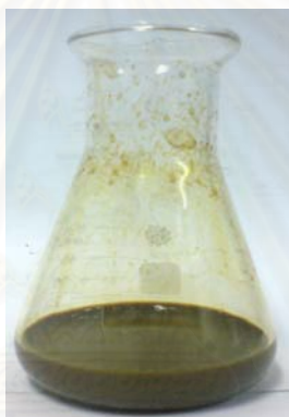
Figure 4.15 The synthesized silver nanoparticles with starch as a stabilizer: highly concentration (10,000 ppm) of silver nanoparticles.
