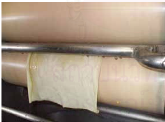
A: Silver-coated cotton fabric was passed through padder.
