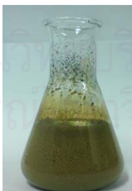
Figure 4.7 The synthesized silver nanoparticles with PVP as a stabilizer: highly concentration (10,000 ppm) of silver nanoparticles.
