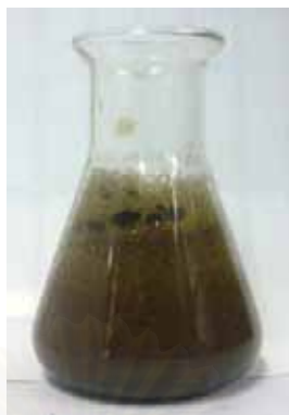
Figure 4.1 The synthesized silver nanoparticles with gelatin as a stabilizer: highly concentration (10,000 ppm) of silver nanoparticles.
