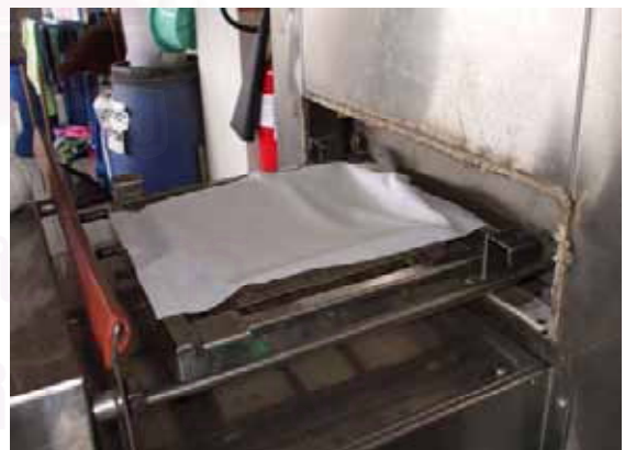
B: Silver-coated cotton fabric in were dried mini dryer.
