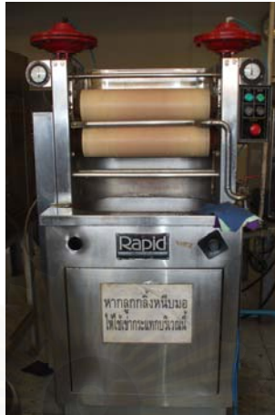
Figure 3.4 Padder (Model P-AO on Rapid brand from Shanghai Colorpilot Electron Co., China).
