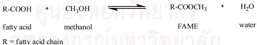
Figure 2.2 Production of fatty acid methyl esters via esterification
