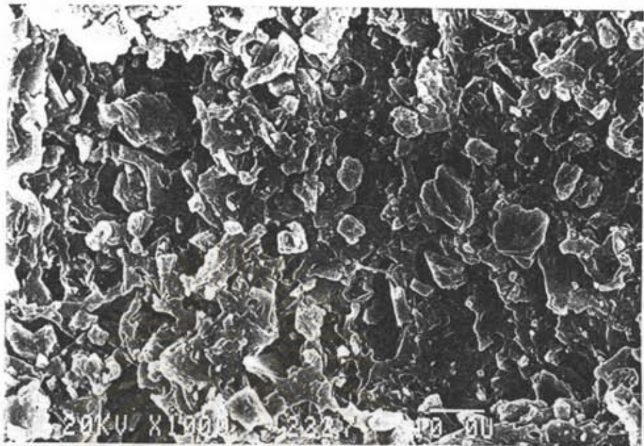
Figure 4.24 Scanning electron micrograph of fracture surface in tear test of \text{CaCO}_3 filled compound at 80:20 ratio of PVC/NBR blends.
