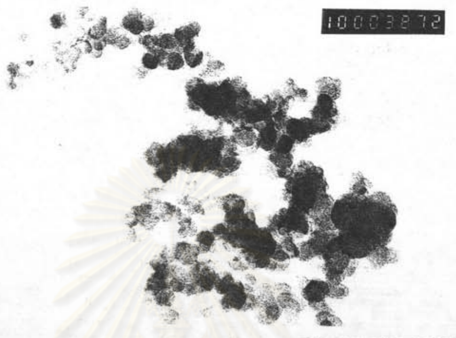
Figure 4.22(a) Transmission electron micrograph of carbon black filler.(x 150,000)
