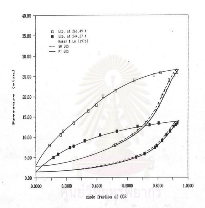
FIGURE 4.2 Comparison of calculated and experimental VLE for  ${\rm CO_2}{\rm -n}{\rm -Propane}$  system
