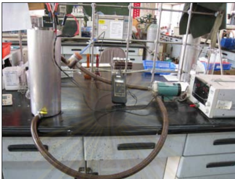
Figure B.1 Electro-Fenton reactor setup.
