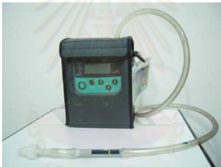
Figure 3.11 The sampling train for the actual sampling
