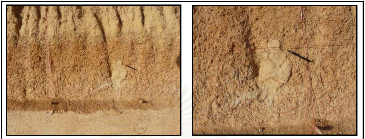
Figure 4.16 Slit lump impregnated in the lateritic layer and the completely weathered rock, the right photograph is a close up silt lump picture at stations 36-37 m.
