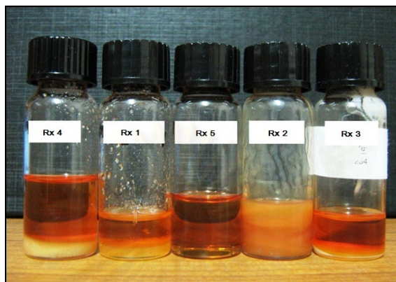
Fig 4.1 Appearance of synthesized molybdate esters after 1 week storage
