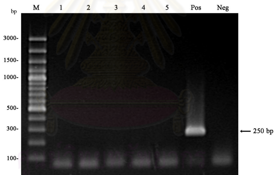
Figure 3.8 Detection of WSSV infection in five individual shrimps. Lane M: 100 bp DNA ladder marker; Lanes 1-5: PCR product of five individual shrimps; Lane Pos: positive control using WSSV as a PCR template; Lane Neg: negative control for PCR reaction. A positive band of 250 bp is shown by the arrow.
