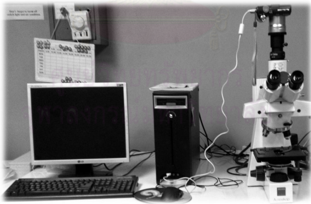
Figure 1 Microscope (Axioskop, Germany) attached with a digital camera (Canon Power shot A640) and conjunction using AxioVs40 V.4.6.3.0 program
