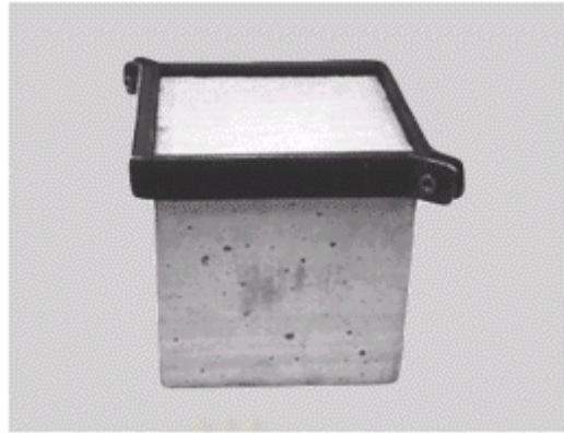
Figure 4.5 : Concrete tighten with a metal frame.
