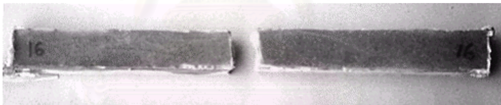
(b) Mortar coated with epoxy composite broke into 2 halves upon impact.
