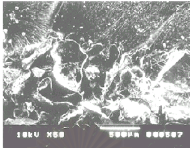
Figure 5.30 : Impact fracture surface in the epoxy layer of the epoxy composite cured at 65 °C for 36 h. The amount of sand added was 27%.
