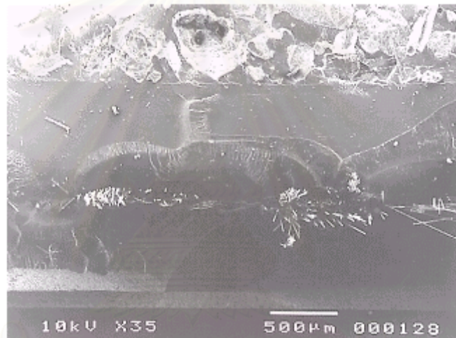
Figure 5.33 : Fracture surface of epoxy composite cured at 65°C 36 h 27% sand.
