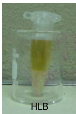
Figure B-2 The color of the ACN extract obtained from each sorbent for the QuEChERS sample preparation using 50 mg each sorbent + 50 mg \text{MgSO}_4 and after the ACN solvent extraction with addition of 500:125 mg \text{MgSO}_4 :NaCl. A blank sample was spiked with steroids at 10 ppm each.
