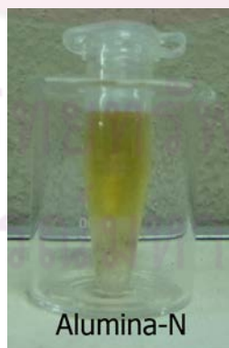
Figure B-2 The color of the ACN extract obtained from each sorbent for the QuEChERS sample preparation using 50 mg each sorbent + 50 mg \text{MgSO}_4 and after the ACN solvent extraction with addition of 500:125 mg \text{MgSO}_4 :NaCl. A blank sample was spiked with steroids at 10 ppm each.
