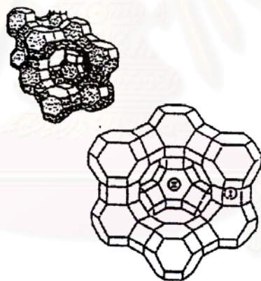
Figure 3.8 Perspective views of the faujasite structure. The silicon or aluminium ions are located at the corner and the oxygen ions near the edges. Type I and II sites are indicated; the supercage is in the center [18].
