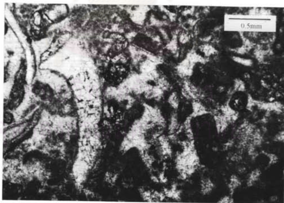
Figure 9 Photomicrograph of Pha Mo Noi sample showing shell fragments with sparry calcite cement.
