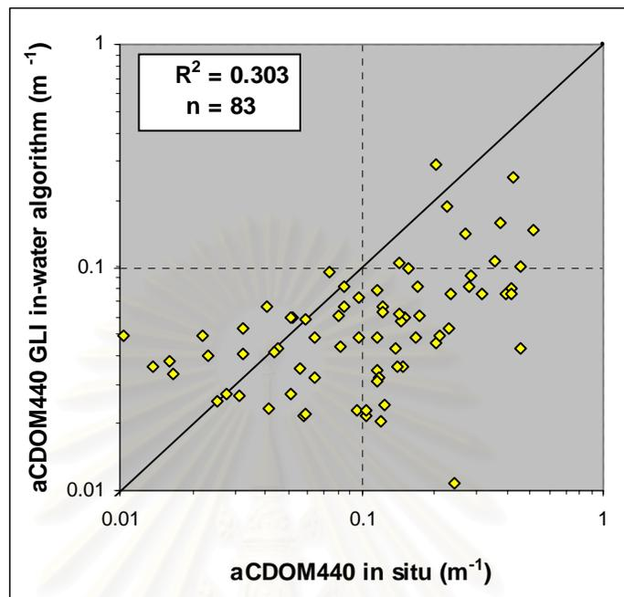
Figure 4.23 Comparison of CDOM observed data and GLI in-water algorithm
