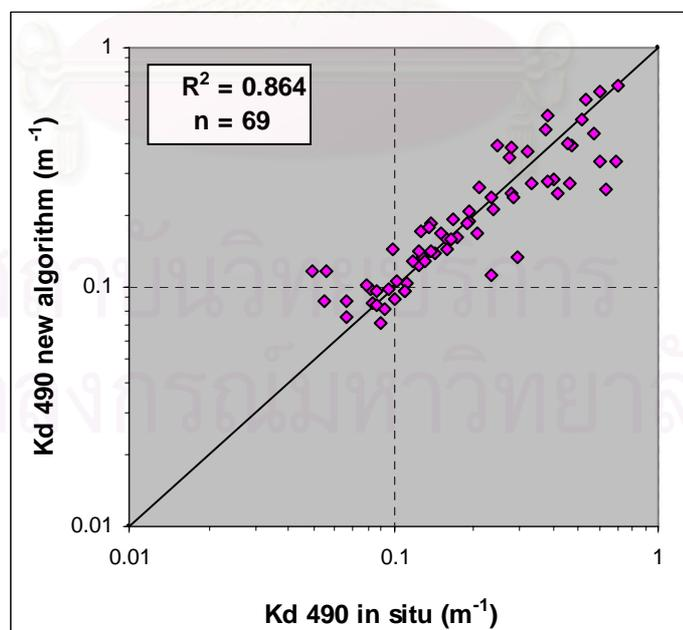
Figure 5.4 Accuracy of the new Kd 490 algorithm
