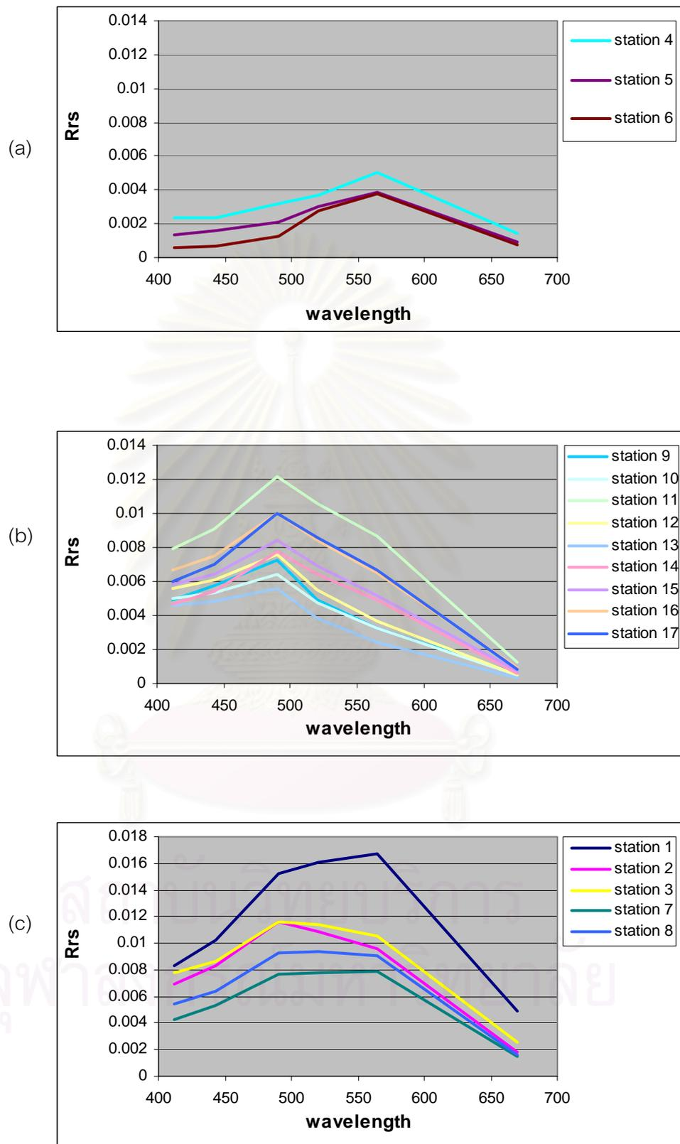
Figure 4.14 Patterns of remote sensing reflectance for cruise 2
