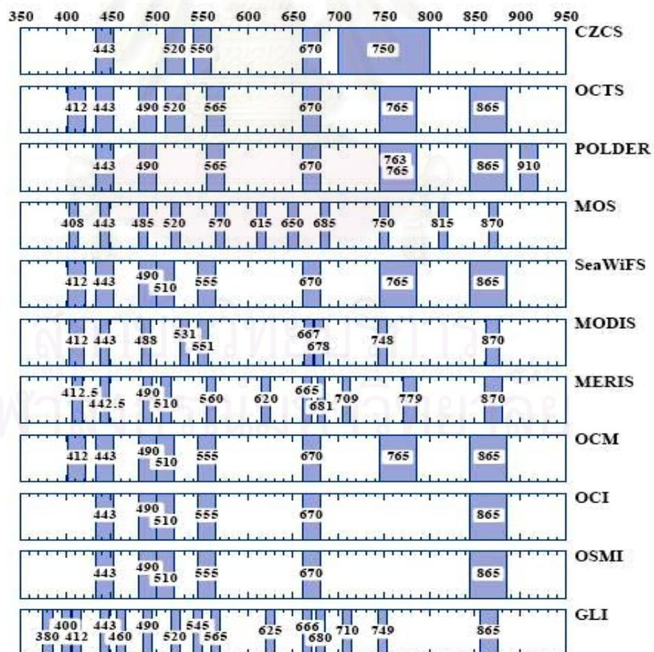
Figure 2.9 Channel positions of various ocean colour sensors (IOCCG, 1998)
