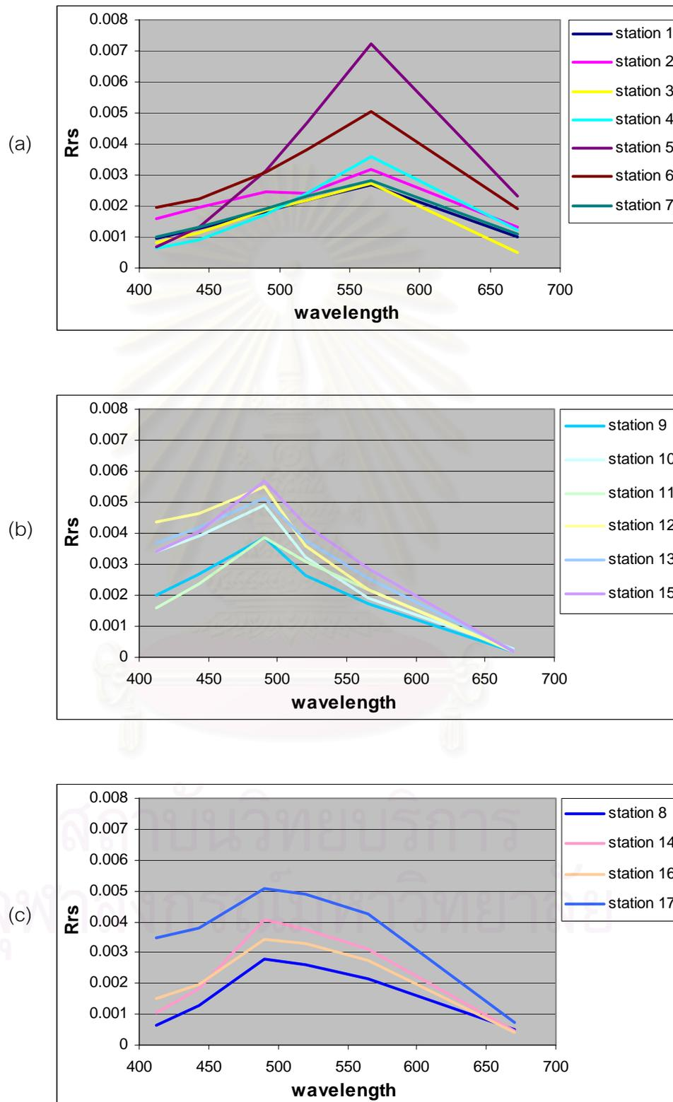
Figure 4.12 Patterns of remote sensing reflectance for cruise 1
