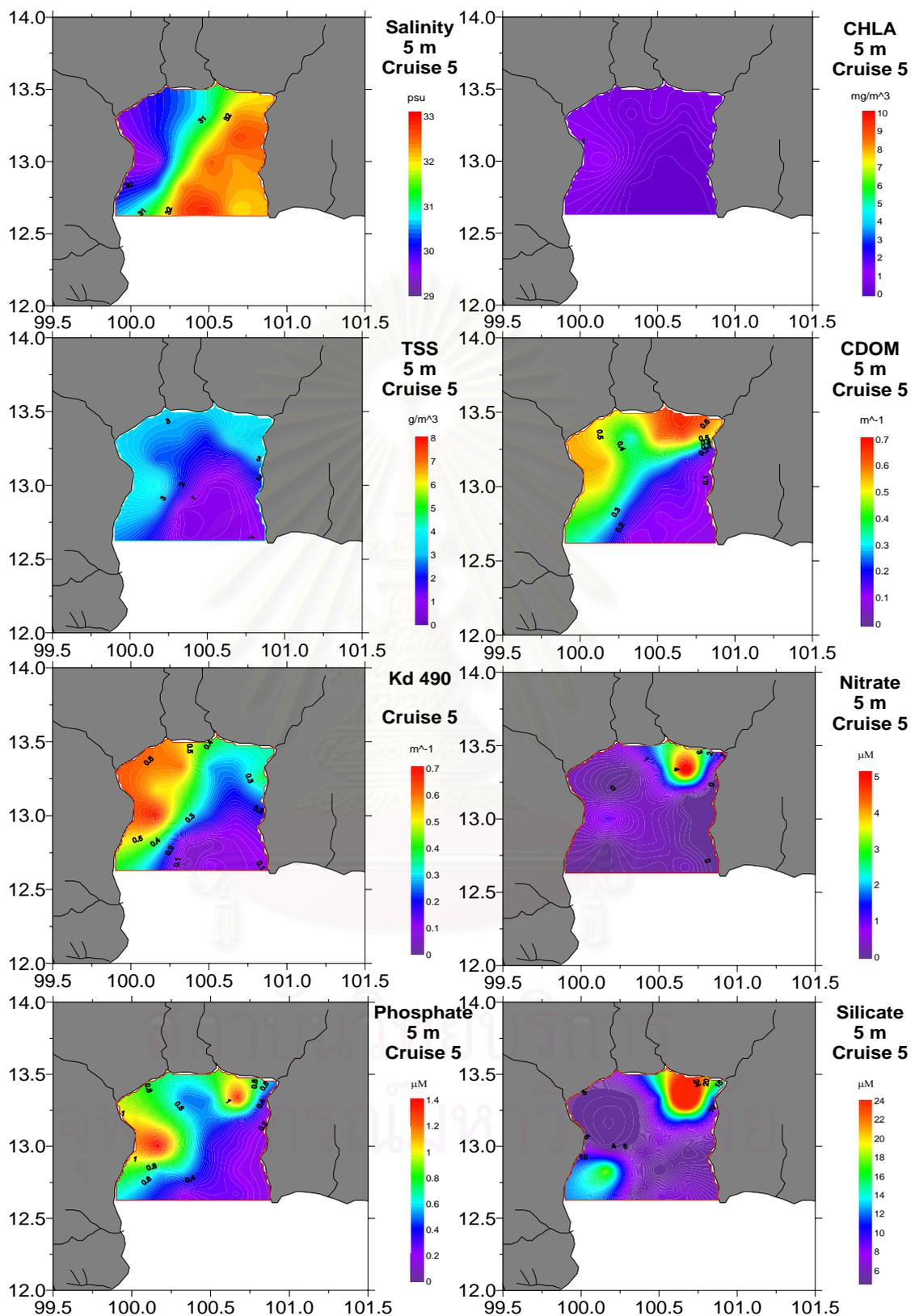
Figure 4.10 Distributions of optically active constituents, salinity, nutrients and  $K_d$  490 at 5-meter depth in cruise 5 (7-10 October 2004) by Kriging interpolation.
