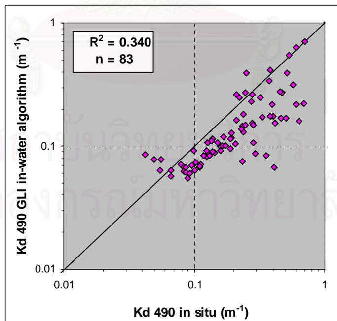
Figure 4.24 Comparison of Kd490 observed data and GLI in-water algorithm
