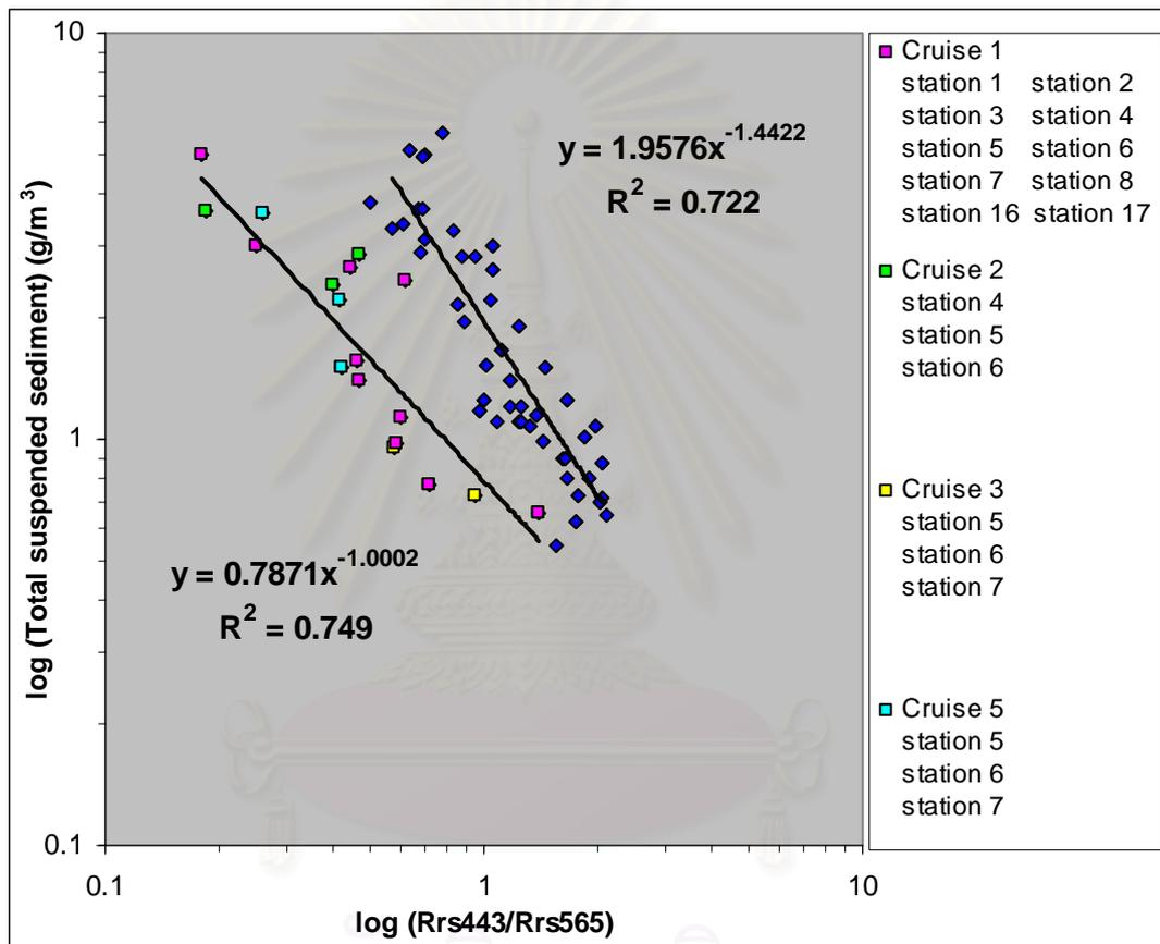
Figure 5.7 Relationship between total suspended sediment and Rrs443/Rrs565. It can separate two optical types of organic and inorganic suspended sediments.
