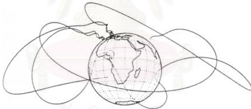
Figure 2.5: A simulated cosmic ray orbit, representing the effect of the Earth's magnetic field on incoming charged particles. The chaos of each orbit depends sensitively on the particle's rigidity and direction of travel. Some particles spiral around the Earth many times before descending to a low altitude. (Source: Friedlander, M. W. Cosmic Rays , 1989)
