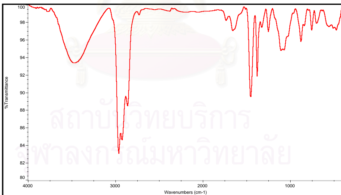
Figure 4.3 FT-IR spectrum of ENR
