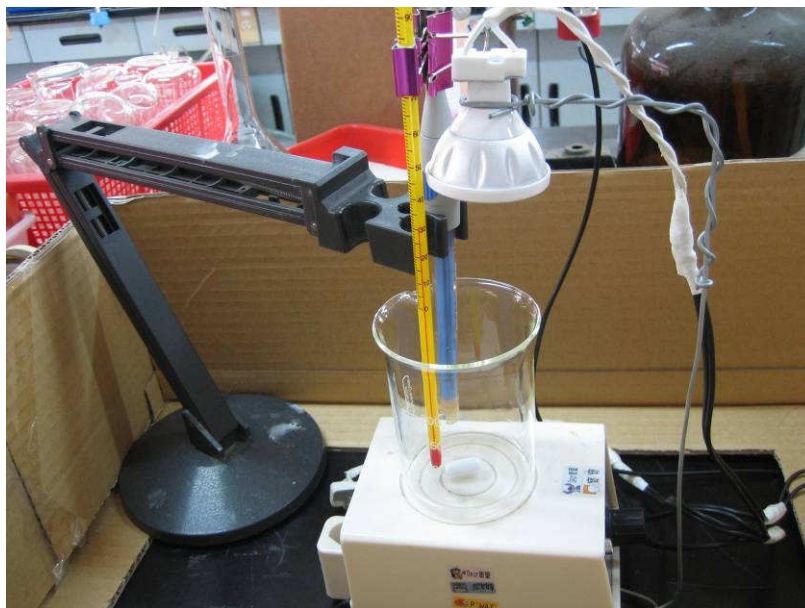
Figure A.1 Reactor Setup (one lamp).
