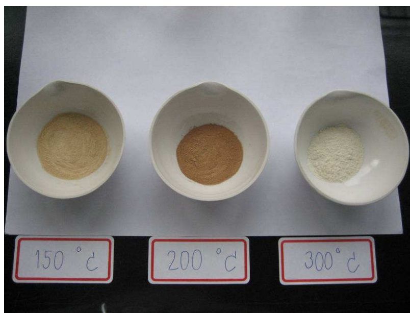
Figure A.3 The color of synthetic TiO 2 at different temperature.
