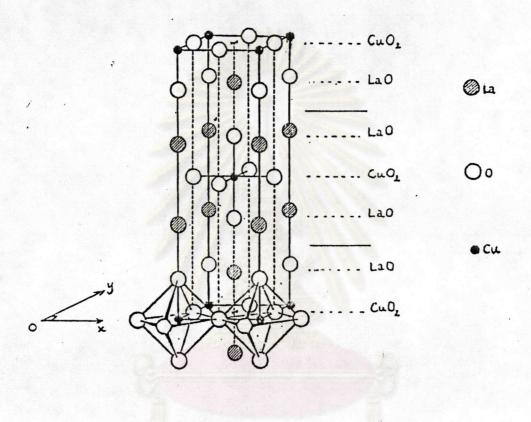
Fig. 1 The layered perovskite K2NiF4 structure
