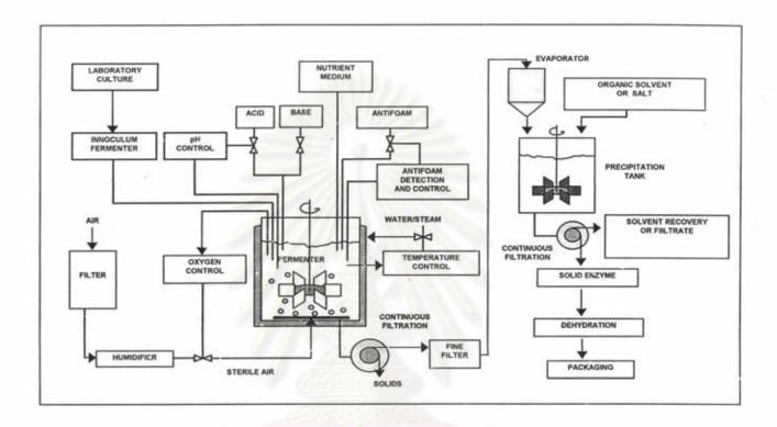
Figure 2-1 Flow diagram for commercial production of microbial protease
