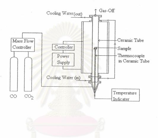
Figure 4.2 Schematic of the Vertical Tube Furnace
