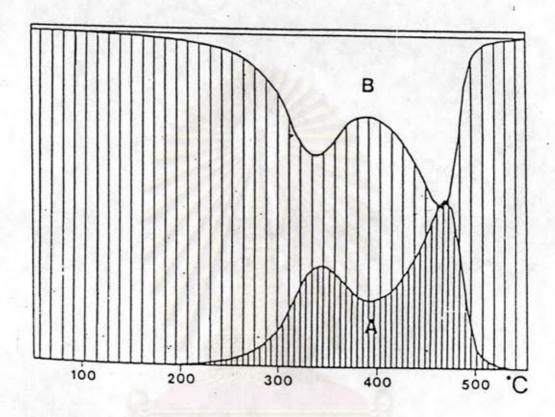
Figure 2.1 Temperature-Programmed Oxidation of coked Pt/Al<sub>2</sub>O<sub>3</sub> catalyst
