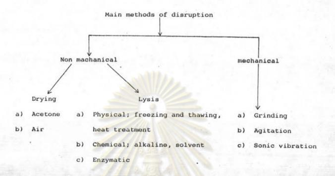
Figure 3-1 Types of non mechanical and mechanical cell disruption
