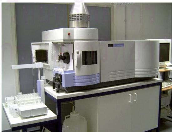
**Fig. 6** Inductively coupled plasma optical emission spectroscopy (ICP-OES: Optima 4300DV, Perkin Elmer Inc., USA)
