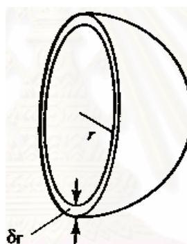
Figure 2.2 Radial distribution functions use a spherical shell of thickness \delta r .
