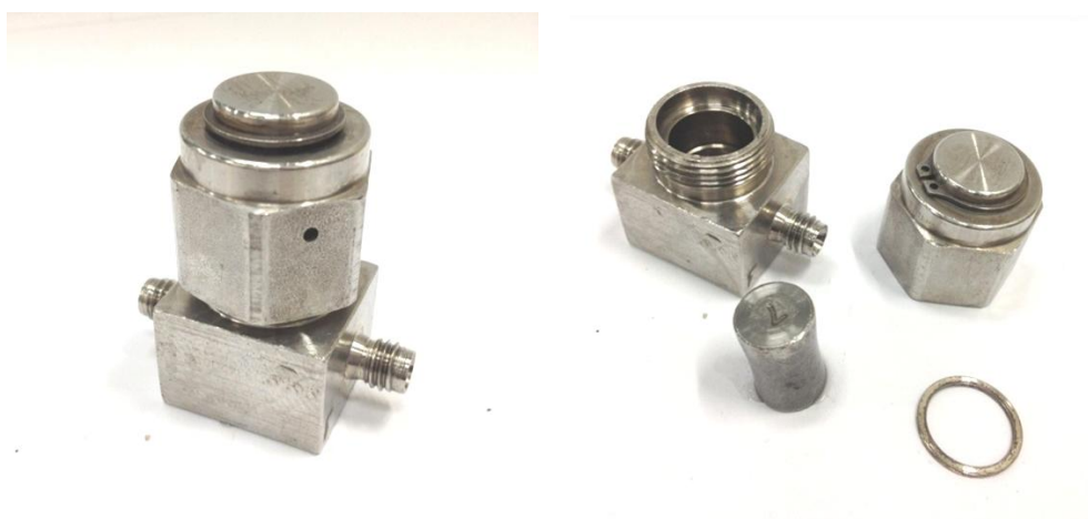
Figure 4.7 The picture of filter separator
