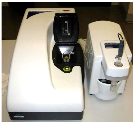
Figure 3.7 Zetasizer (Malvern, Nano – ZS: model ZEN 3500)
