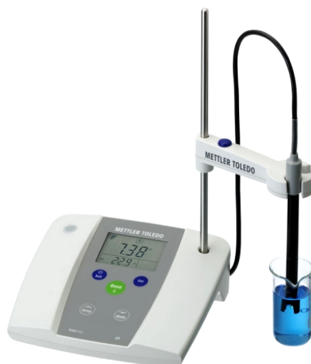
Figure 3.8 pH meter (Mettler Toledo, Five Easy model FE20)
