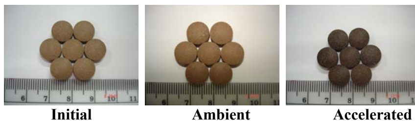
Figure 16. The appearance of core tablets after freshly prepared and storage conditions for 4 months.
